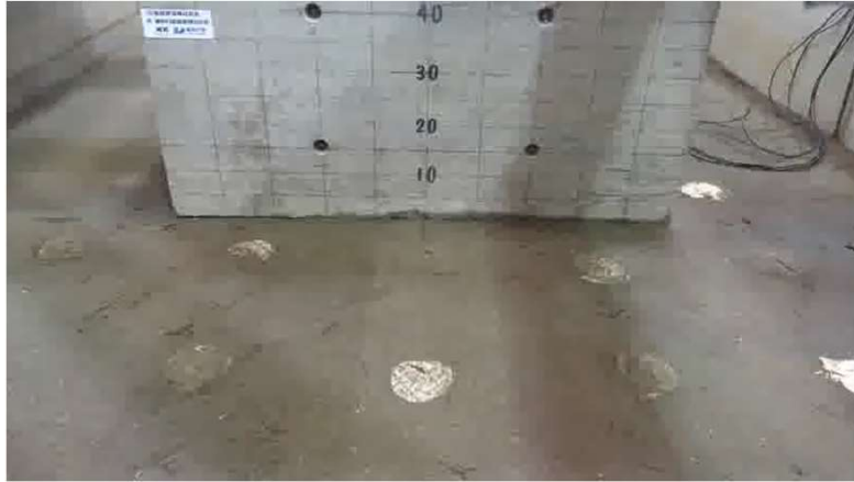
Input motion : 150 Gal (165 Gal) Improvement method : Log pilling, Pitch = 4D(丸太打設地盤)
